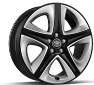
17-in. 5-spoke alloy wheels with titanium-finished wheel inserts
