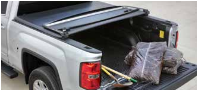
TONNEAU COVERS The soft cover shields cargo and easily rolls up to allow full access to the bed and is constructed with integrated crossbows. A soft tri-fold cover is also available. The hard cover is tri-folding and adds strong content protection and easy access to the cargo box. All three covers display a GMC logo.
