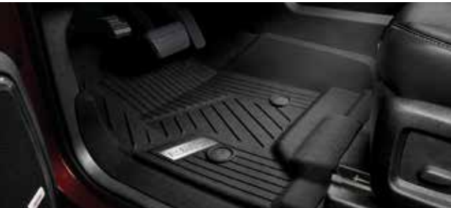
PREMIUM FLOOR LINERS Sierra's floor liners take all-weather floor mat coverage further with raised edges to help protect floor and trim contours.
